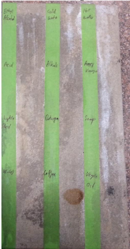
Photo 3 – ASTM D1308 – Staining Test – After to Testing
